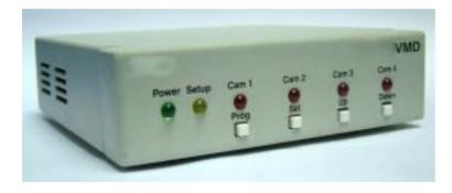
The VM D1004 is a 4 camera video switcher that has VMD (Video Motion Detection) on each camera. OSD (On-Screen) programming for switching dwell time, bypassing and motion dwell time along with the VMD setups is all done via 4 front panel pushbuttons. Independent defined motion areas and sensitivity for each camera. One video output will be able to drive two 75 ohm video loads at 1VP-P. One hard alarm output is provided whenever any camera goes into motion alarm mode.
